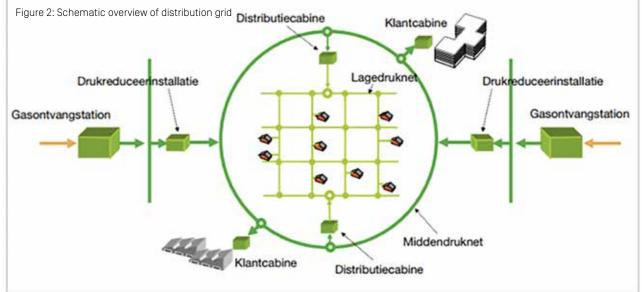
Distribution grid pressure is divided into different pressure classes:
