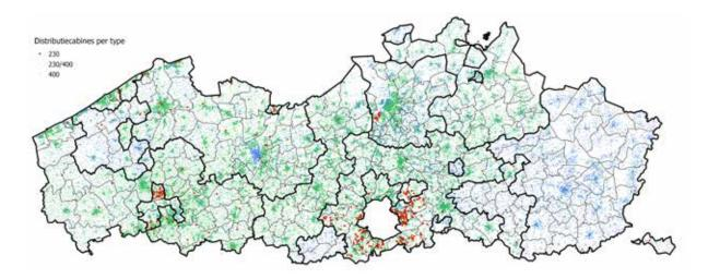
Figure 10: Concentration of distribution cabins capable of supplying 230V, 230V/400V or 400V. For historical reasons, these cabins are mainly located on the outskirts of Brussels.
