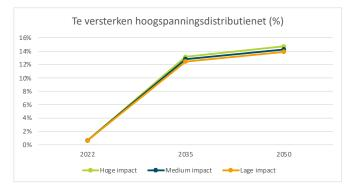
Note that part of the high-voltage distribution grid to be enhanced consists of cables at less than 100% load. This is a result of the redundancy designed on the highvoltage distribution network. In the event of an incident [such as a cable failure], it can be re-switched to re-feed as quickly as possible and reduce prolonged high-impact incidents.
