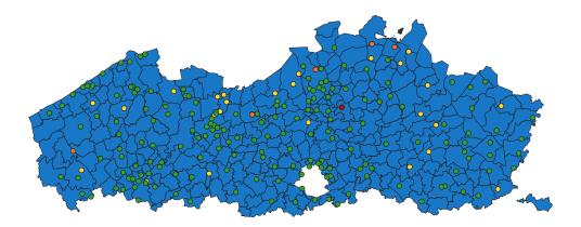
Figure 12: Interconnection point load in injection (green < 25% load, yellow 25%-50% load, orange 50%-75% load)
