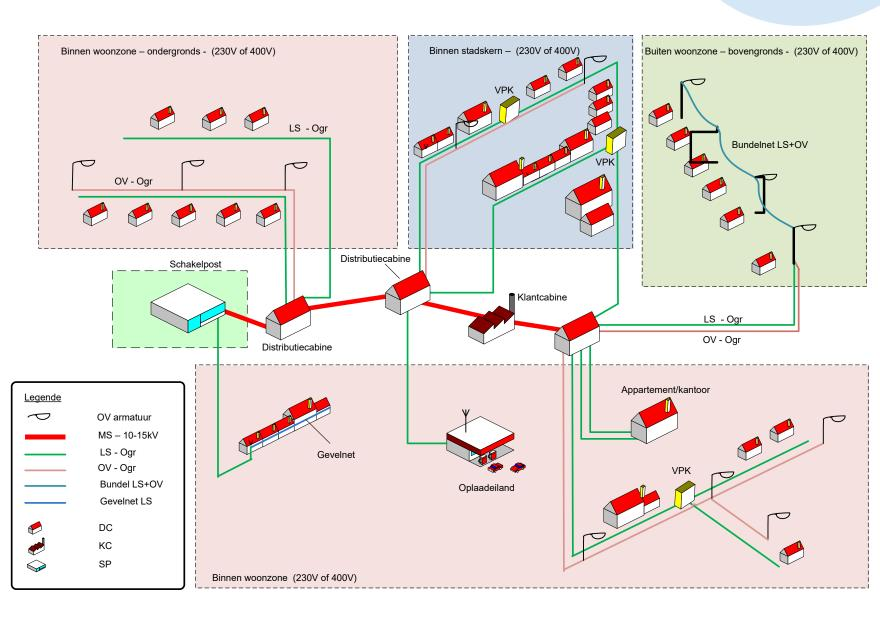
A high-voltage distribution loop starts from the switching station. Distribution cabins and customer cabins are successively connected to the same high-voltage distribution grid. The distribution loop usually terminates at the same switching station, or one nearby.
