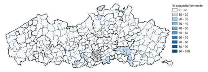
On top of the current network state, we simulated additional grid loads according to a high, medium and low-impact scenario. The low-voltage electricity scenarios are mainly determined by the increase in home charging for electric vehicles and the increase in heat pumps for residential heating, considered at the time of the (winter) evening peak. The scenarios examined are:
