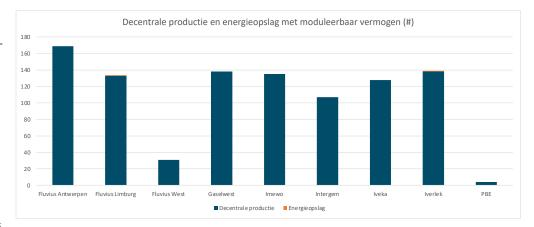
Fluvius provides a remote control cabinet at facilities for decentralised production and energy storage systems with a capacity > 1MVA or at smaller facilities in the event of potential grid congestion, see TRDE Art. 2.2.54. In Fluvius' operational area, there are 1,303 production installations (total installed capacity 3GVA) and 4 energy storage systems where adjustment of facility capacity is possible. Below is a summary of the modulations of these facilities over the past two years:
