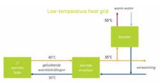
Finally, heat sources that cannot be used directly for space heating, nor for the production of domestic hot water are categorised as 'very low temperature'. For heating purposes, these sources can provide input to the evaporator side of a heat pump, but they can also absorb heat as part of active or passive cooling systems. Thus, they allow energy exchange in two directions and therefore the associated grids work fundamentally differently from classical heat grids.
