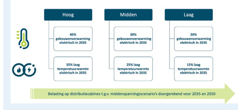
We also calculated the load on distribution cabins resulting from the 2035 and 2050 low-voltage scenarios at high-voltage, adding the impact of electrification of heating and low-temperature process heat for professional customers.
